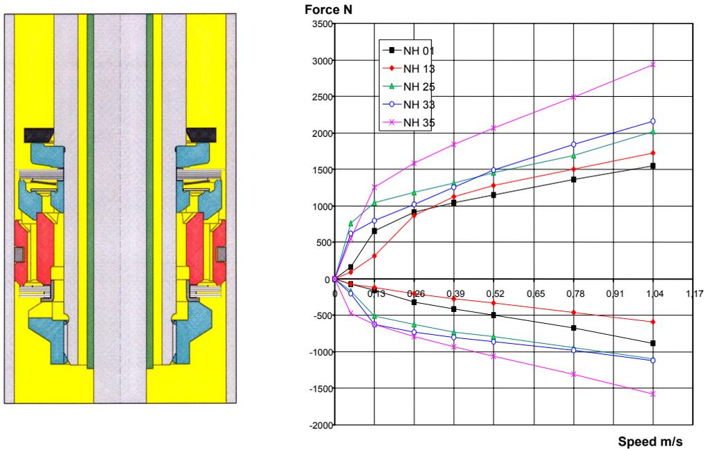
Fig. 7: Design of characteristic curves with "comfort piston"
