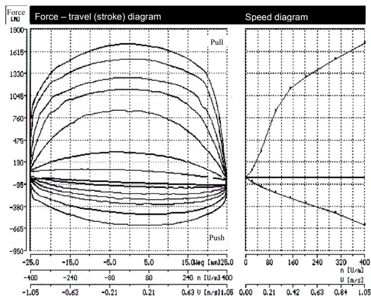
**Fig. 6: Nivomat damping curves**
