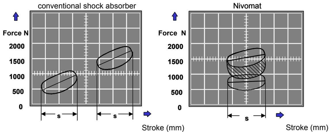
Fig. 8: Load-sensitive damping
