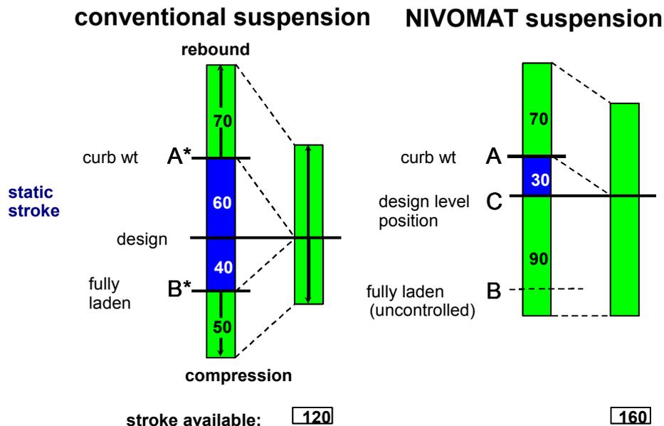
**Fig. 4: Nivomat stroke in comparison with conventional damper**
