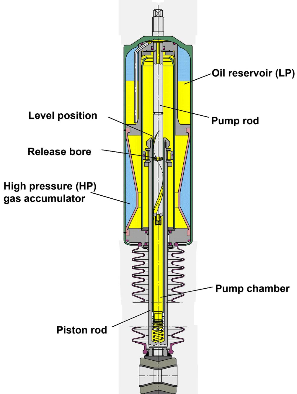
**Fig. 2: Nivomat – structural design**
