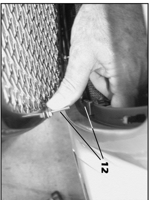
12. Align the E&G Mesh Grille's middle mounting studs with the factory enlarged mounting holes in the bumper cover before you align the upper mounting studs with the enlarged factory mounting holes.
