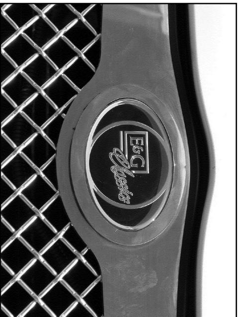
15. For all grilles: Make sure to thoroughly clean the emblem recess with alcohol to remove grease and fingerprints. Peel the backing from the E&G emblem and install the emblem in the center of the E&G emblem surround.
