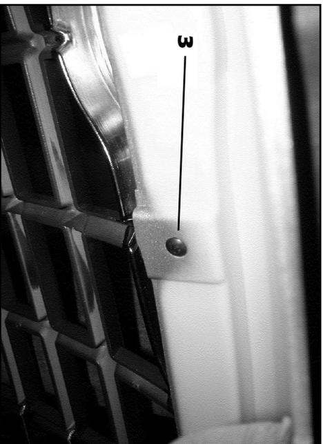
3. Remove the four (4) factory fasteners (#2 square drive bit) across the top and one (1) down each side of the grille.
