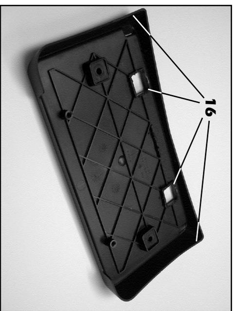
16. Trim the front tag bracket (if equipped), removing the top mounting bosses and trimming the left and right extensions that originally fit into the front grille opening recess. When finished, the modified tag bracket should look this this.
