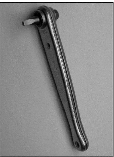
5. The best way to remove the lower four (4) factory mounting screws is to use a small ratcheting screw driver or a ratcheting box wrench and a #2 square drive short bit (as shown). The large plastic screws that secure the bumper cover to the black bumper styro-foam need to be removed using a #3 square drive bit (not shown).
