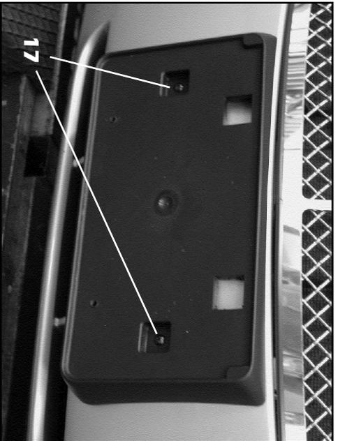
**17.** Align the modified front tag bracket below the mesh grille (where shown). Install the modified tag bracket back onto the bumper cover by drilling new 3/32" mounting holes and reusing the factory screws (**DO NOT OVERTIGHTEN**). Reinstall the radiator support panel cover (not shown).
