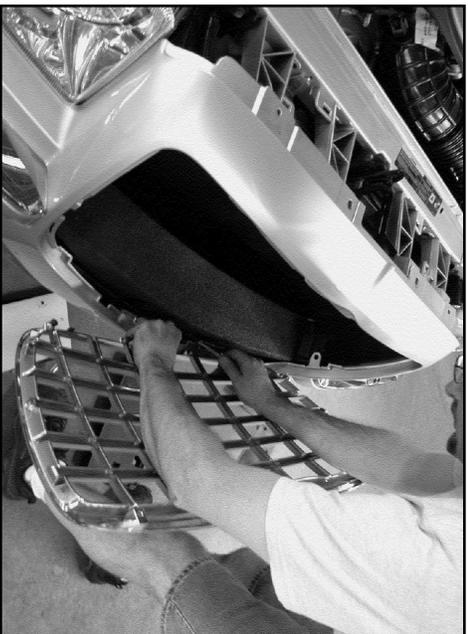
6. Remove the lower four (4) securing screws by pulling the grille out as far as you can to gain clearance for screw removal. Remove the screws from left to right, the subsequent screws will be easier to remove as you will be able to pull the grille farther out.
