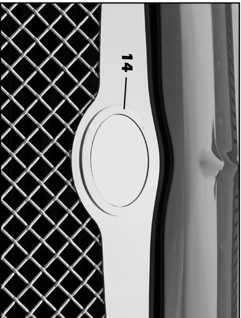
14. For "Heavy Mesh", "Euro", "Center Bar" & "Double Mesh" grilles only: Clean the top of the stainless surround and emblem surround with alcohol to remove grease & finger prints. Install the supplied double faced tape ring to the back of the emblem surround. Align the E&G emblem surround. Peel back a small section of the double faced tape backing, align the emblem surround, pull out the tape backing and press the emblem surround firmly into place.
