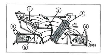
The outside (fresh) air intake can be shut off by selecting the Recirculation Mode with the mode control. This will operate an electrically actuated recirculation-air door (4) that closes off the fresh air intake and recirculates the air that is already inside the vehicle.
